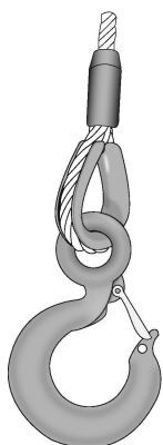
Eye Sling Hook With Latch & Thimble
