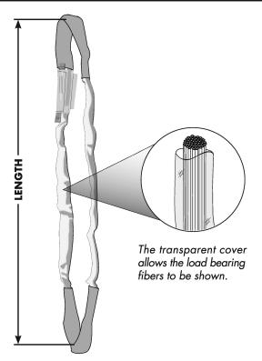
**FIRST®** High Performance RoundSlings supply riggers with a consistent and reliable visual inspection. **FIRST®** High Performance RoundSlings use a transparent cover that embodies and protects the load bearing core yarns without prohibiting a visual inspection of the working roundsling.
